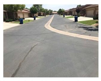
This component includes a provision to pulverize the existing asphalt, removing excess materials, grade and compact pulverized material, and repave with 2.5" of new asphalt.
