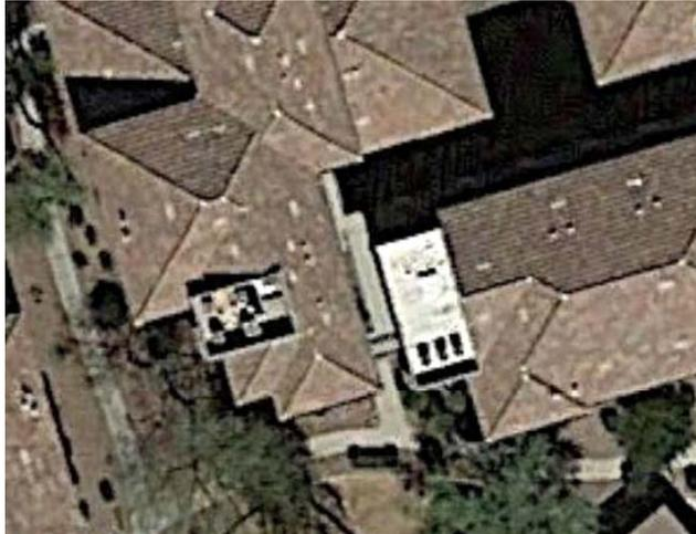
In February 2016, \$1,080 was spent to clean, repair and apply a silicone top coating to one (1) flat, A/C equipment well roof. In mid-2016, \$10,591.76 was spent on similar work to 11 flat, A/C equipment well roofs. This component budgets to recoat these 12 flat roof areas on a 10 year cycle. AV Builder & the client should have records of which 12 roofs this component is for.
