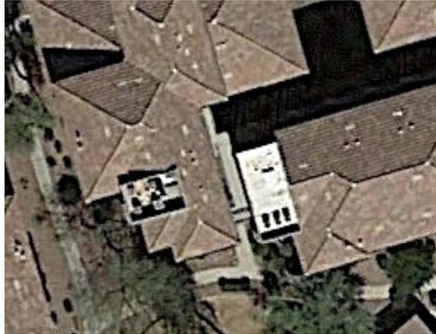
There are 104 flat, A/C equipment well roofs atop various buildings. In 2012/2013, 92 of the flat, A/C equipment well roofs were cleaned, repaired and received a new, silicone top coat application. This component budgets to recoat these 92 flat roofs on a 10 year cycle.
