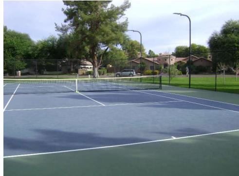
Good condition. Budget to resurface two tennis courts. No anticipation to replace courts. Replaced in 2018 with post tension concrete total \$86,000. Noted no cracking. Resurfaced approximately 2-3 years ago.
