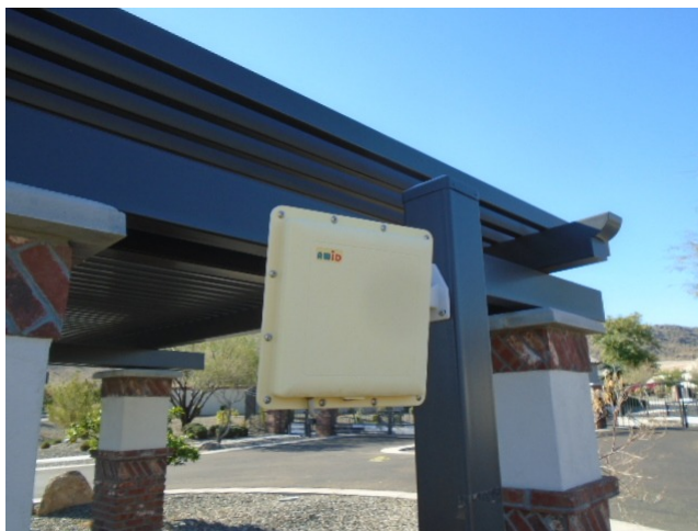
This is an Applied Wireless ID, LR-3000 RFID reader.
