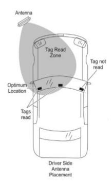
Tags must be installed a minimum of 2.5" from any metallic material, including the rearview mirror. If installing on the outside of the vehicle, ensure the tag is clear of the windshield wiper path.
